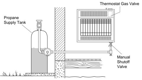
Figure 16 - Checking Gas Joints
